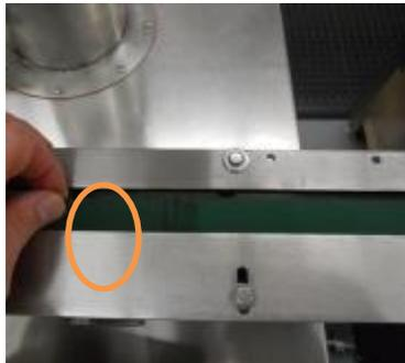
**Electrical Cable In Contact With Rotating Gear**
