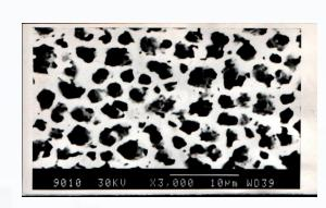
Polymeric blend membranes (for Desalination)
