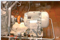
Figure 2. Overheated gearbox: (a) visual, (b) infrared
